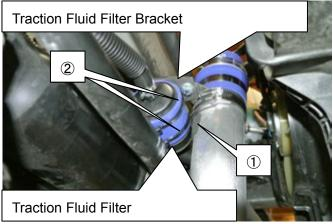
(51)Secure the Hose 22mm assembly to the Suction Pipe No.1 using ①Hose Clip 22mm.
