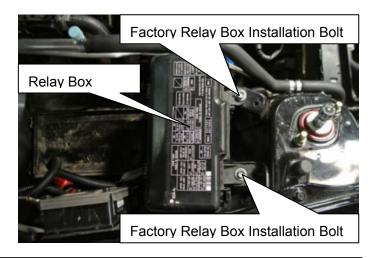
(18) Install ①Relay Box Bracket No.1 to the relay box.
