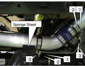
(32)Install the Relief Valve Assembly to the Intercooler Outlet Pipe No.3 after inserting the gasket of the Relief Valve Assembly between the pipe and valve.
