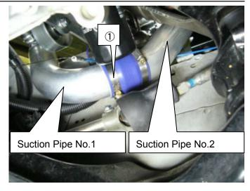
(19) Affix the provided Sponge Sheet to the portion where the Suction Pipe No.1 may come in contact with the Intercooler Inlet Pipe No.1.
