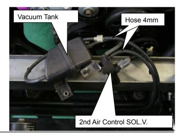
(34)Install the 2nd air control solenoid valve and vacuum tank to the vehicle using ①Hexagon Bolt M6 L=25, ②Large Diameter Washer M6, and ③Spacer M6 L=3
