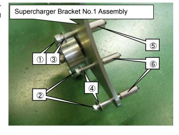
(28)Temporarily install the assembled Supercharger Bracket No.1 to the Supercharger Bracket No.2 using ⑦Cap Bolt M10 L=25 (P1.5) and ⑧Washer M10.
