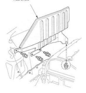
(13) Remove the exhaust manifold cover.
