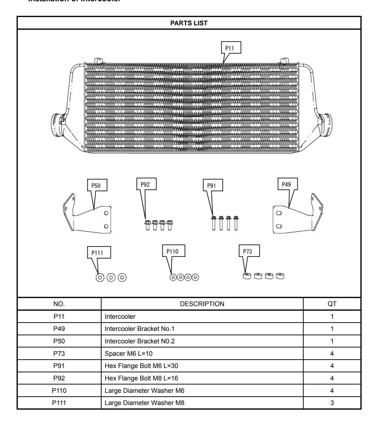
(1)Temporarily install the Intercooler Bracket No.1 and No.2 to the Intercooler using ①Hex Flange Bolt M8 L=16, and ②Large Diameter Washer M8.
