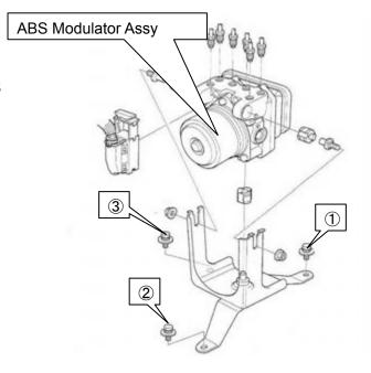
(41)Install ④ABS Modulator Bracket, ⑤Large Diameter Washer M6, ⑥Nut M6, and ⑦Spacer M6 L=3 to each position of the bolt ① and ② removed in (24) as shown in the diagram below. Reinstall the bolts ① and ② to secure them to the vehicle. Relocate the ABS Modulator Assembly to the right side of the vehicle.
