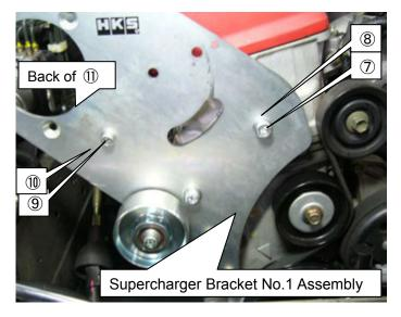
(30)Tighten the Supercharger Bracket No.1, No.2, and No.3 to the final tightening torque. Make sure to tighten them properly.
