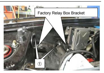
(21) Install the relay box assembly to the vehicle using ①factory relay box bracket fixing bolt.
