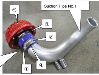
(18) Install the Suction Pipe No.1 to the Suction Pipe No.2 using ①Hose Clamp #36.
