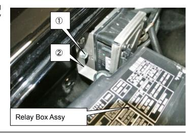
(23) Install the relay box assembly to the vehicle using ①factory relay box bracket fixing bolt.
