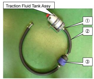
(10)Install the Traction Fluid Tank assembly to the vehicle using the following provided parts.
