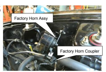
(12)Loosen the factory bolt on the center of the horn.
