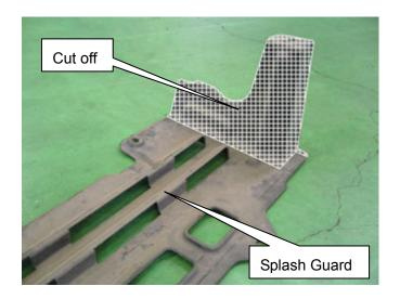
(69)Cut off the shaded portion of the front bumper so it does not come in contact with the intercooler.
