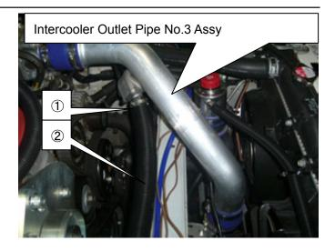
(48) Adjust the position of the Intercooler Outlet Pipe No.1, No.2 and No.3. Tighten the bolts and hose clamp securely.
