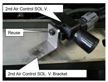
(32)Remover the 2nd air control SOL.V.vacuum tank from the vehicle.
