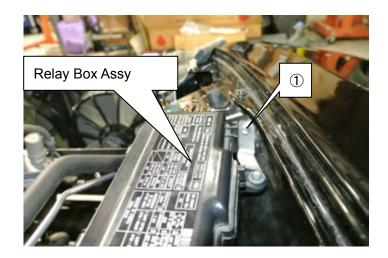
(22) Remove ①factory EPS control unit fixing bolt. Install the relay box assembly to the vehicle using ②Relay Box Bracket No.3 and ①.
