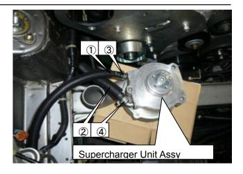
(38)Install the Supercharger Unit to the Supercharger Bracket No.1 using ①Dish Bolt M8 L=35.
