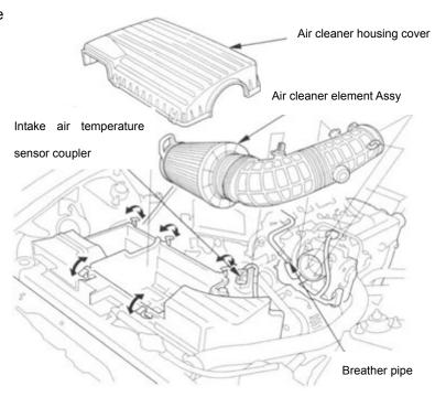
(10) Remove the intake air temperature sensor harness clamp and air cleaner housing.
