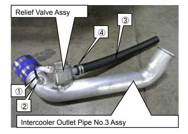
(39)Install ③Hose 22mm L=380mm and ④Hose Clip 22mm to the Relief Valve assembly.
