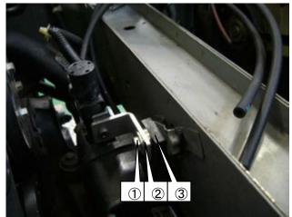
(35)Replace the breather pipe assembly with ①Joint Pipe 8mm.
