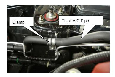
(25)Bend the thick A/C pipe to avoid unnecessary contact with the Supercharger unit and other parts.
