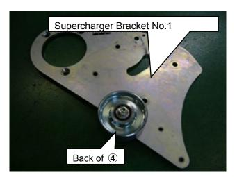
(7)Install the Idler Pulley to the Tensioner Bracket using ①Cap Bolt M10 L=50, ②Washer M10, ③Spacer M10 L=7.5, and ④Flange Nut M10.
