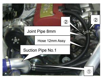
(54)Secure the Hose 12mm assembly to the Hose 22mm assembly using 1Tie Wrap(L), 2Tie Wrap(M), and 3Tie Wrap(S).
