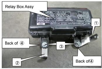
(20) Remove ①factory relay box bracket installation bolt; then, remove the factory relay box bracket from the vehicle.
