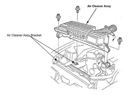
(9)Remove the intake air temperature sensor coupler and breather pipe; then, remove the air cleaner housing cover and air cleaner element assembly.
