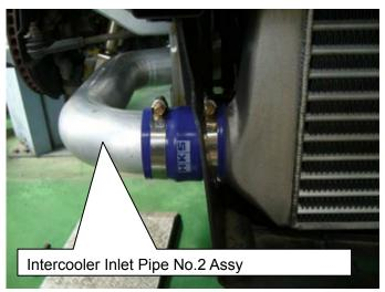
(15)Adjust the position of the Intercooler Inlet Pipe No.1 and No.2. Tighten the bolts and hose clamps securely.
