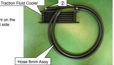
(12)Install ④Traction Fluid Cooler Bracket No.1, ⑤Traction Fluid Cooler Bracket No.2, and ⑥Traction Fluid Cooler Bracket No.3 to the Traction Fluid Cooler Assembly using ①Hexagon Bolt M8 L=15, ②Large Dia. Washer M8, and ③Flange Nut M8.
