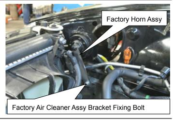
(14) Remove the vinyl tape from the factory horn coupler's end and install the factory horn coupler to the factory horn that was relocated.
