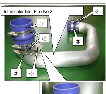
(13)Temporarily install the Intercooler Inlet Pipe No.2 assembly to the vehicle.
