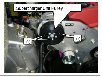
(43)Install the provided Belt as shown in the diagram on the right.
