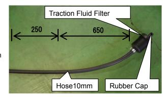
(4)Cut the Corrugated Tube 8mm to 950mm and 1300mm. Cover cut Hose 8mm with the cut Corrugated Tube.
