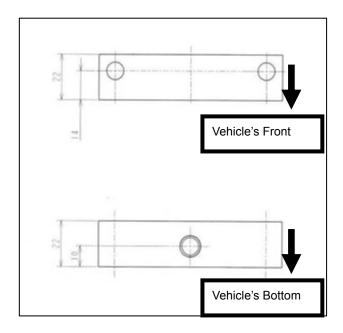
(9)Temporarily install the Supercharger Bracket No.3 to the spool solenoid valve using ①Cap Bolt M6 L=60 and ②Large Diameter Washer M6.
