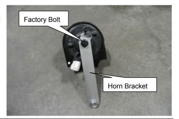
(13) Install the factory horn assembly to the vehicle using ①factory air cleaner assembly bracket fixing bolt.
