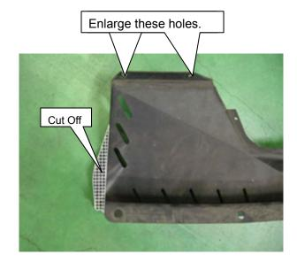
(16)Enlarge two holes on the front air guide to 11mm. (See the diagram on the right.)
