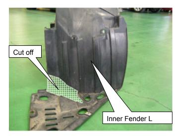
(68)Cut off the shaded portion of both sides' splash guard so they do not come in contact with pipes.
