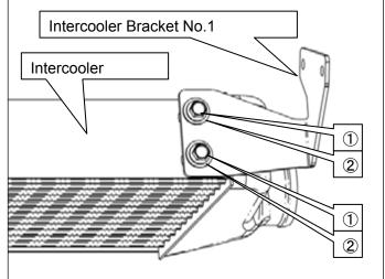
(2)Install the Intercooler assembly to the vehicle using ① Hex Flange Bolt M6 L=30, ②Large Diameter Washer M6, and ③Spacer M6 L=10.
