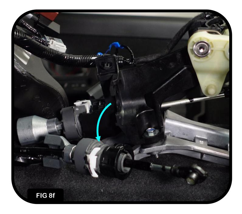
STEP 8 Cont. - Remove Shifter Cables From Shifter
