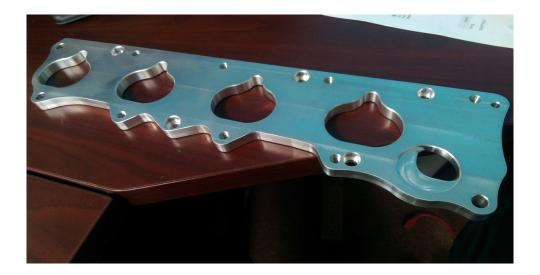
Thank you for purchasing the JSP K24/F20 S2000 intake adapter. These instructions will go over the basic installation and modifications required to your S2000 intake manifold and K24 cylinder head for proper installation. This installation is recommended to be done by a professional, if at any point you do not feel that you are capable of completing these steps, please consult your local fabrication or machining shop.
