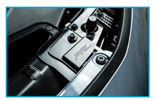
16. Attach the PRL 4" air filter onto the PRL High Volume MAF housing. Use the worm gear clamp, tightening firmly. Align the MAF on the side of the airbox.
