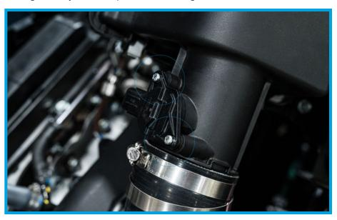
21. Once the MAF sensor is in place, re-attach the MAF harness to it. Check all other connections to ensure everything is tight and in place.
