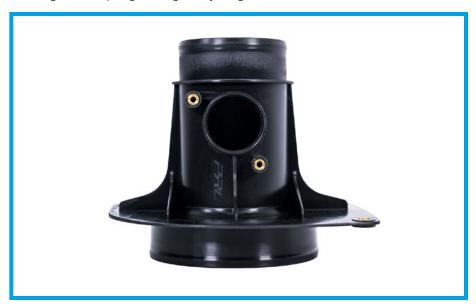
17. Using the (3) provided M5x10mm button head screws, use a 5mm Allen wrench to attach the MAF housing to the PRL High Volume airbox. Do not overtighten, as you can crack the rotomold material.
