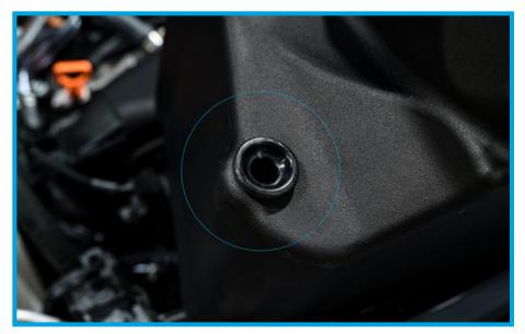
14. Place the PRL HVI Airbox into the engine bay, seating it on the factory and PRL mounting post. Tighten the (1) factory 10mm bolt on the right side of the airbox.
