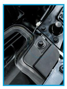
5. You will also need to remove the (1) plastic tab that affixes the factory air duct. You can use a flathead screwdriver to remove. This will not be re-used.
