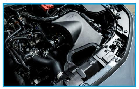
18. Place the Silicone Intake Hose and (2) worm gear clamps onto the MAF housing and the factory inlet. Adjust to where the PRL logo is facing upwards.
