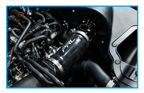
19. Once the silicone is adjusted properly. Tight to the (2) worm gear clamps. They should be snug, but do not overtighten to where the silicone is pinched.
