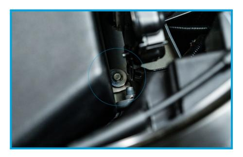
15. Affix the PRL Inlet Duct to the PRL High Volume airbox. Attach with the (3) plastic push rivets. Using the (2) factory 10mm bolts, attach the duct to the core support.
