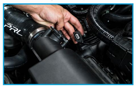
9. Use a 12" extension remove the (1) 10mm bolt on the right side of the airbox. We advise using a magnetic socket/magnetic pick so to not drop the bolt into the engine bay. This will allow the factory air box to be removed.
