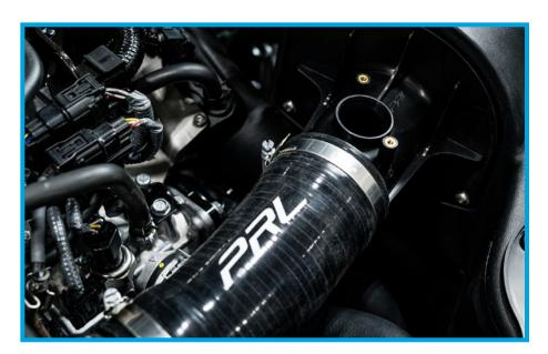
20. Remove the factory MAF sensor from the factory airbox. These (2) factory screws will not be re-used. Insert the (2) provided M4x6mm socket head screws into the PRL MAF housing and tighten using a 3mm Allen wrench. Do not overtighten as you can strip the MAF housing holes.
