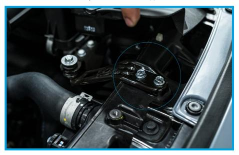
7. OPTIONAL: If you need more clearance to reach the (1) 10mm bolt on the side of the airbox, you can remove the resonator from the factory hose. Simply wiggle it back and forth till it comes free from the hose.
