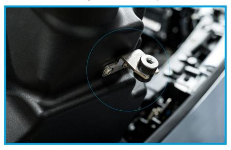
13. The rear of the airbox will have a PRL Rubber Grommet placed into it. This allows you secure the PRL HVI airbox to the mounting post in the engine bay.
