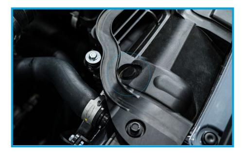
6. Use a 3" extension to remove the (2) 10mm bolts from the bracket on the front of the airbox. You will then remove the (2) 10mm bolts to remove the bracket that holds the factory duct to the core support.
