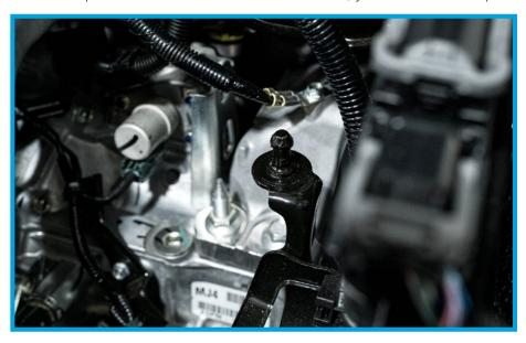
11. Place the Airbox Mounting post in the bracket, with the (1) M6x30mm bolt. Install the provided Mounting Bracket A to the core support with (2) factory 10mm bolts.
