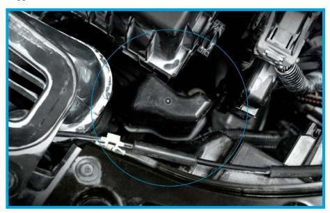
8. If you have not done so, disconnect the MAF sensor harness from the factory MAF sensor. Simply lay the harness out of the way for now. You will take the MAF sensor out of the factory MAF in a later step.
