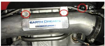
4: Remove the two 10mm bolts holding the wire harness shown in red circles. Remove the two 14mm bolts shown in white circles that attaches the inlet housing to the compressor side. Unplug the wire harness for easier access to one of the 14mm bolts. An extension will be needed for this, preferably with a swivel head. Various lines may need gently held out of the way to access all of the bolts.
