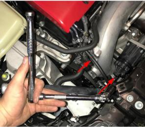
5: Install the PRL cast aluminum inlet section by reusing the two 14mm bolts that connect to the compressor inlet along with the stock black metal gasket. Note orientation of the stock gasket on the stock piece. Reinstall two 10mm bolts for the wire harness. Re-install the wire hardness and install the PRL silicone adapter with the hose clamp on the casting side. Make sure to push the coupler fully on until it meets the stopper inside.
